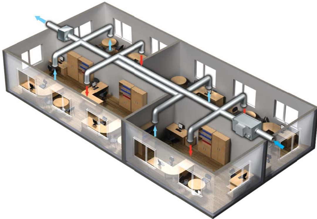
MPA unit office air exchange example.
