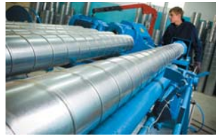
Spiral air ducts workshop
